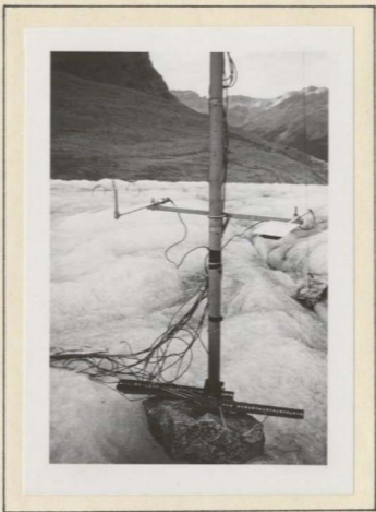
Figure 2.2 Wind velocity and temperature sensors near the ice surface
