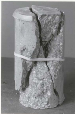
Figure 5.1: A high strength concrete cylinder at failure
