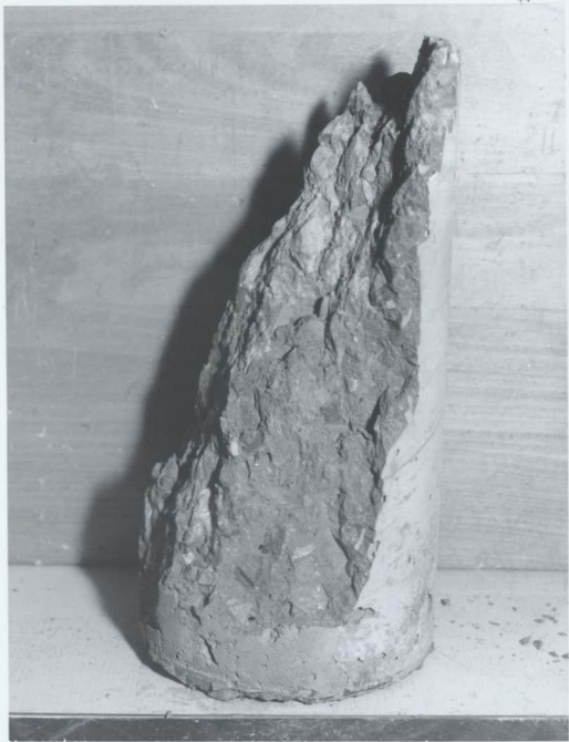
Figure 3.2: Failure surface of a high-strength concrete cylinder
