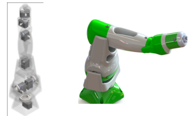
Fig. 4. Design of Anthropomorphic robot with 5 DoF
