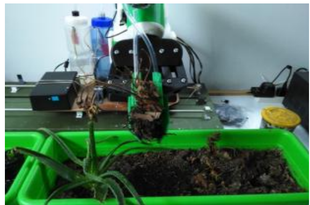
Fig. 34. Process of weeding or removal of plants.
