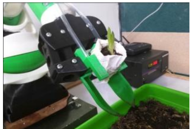
Fig. 35. Realization of the sowing process by transplant.
