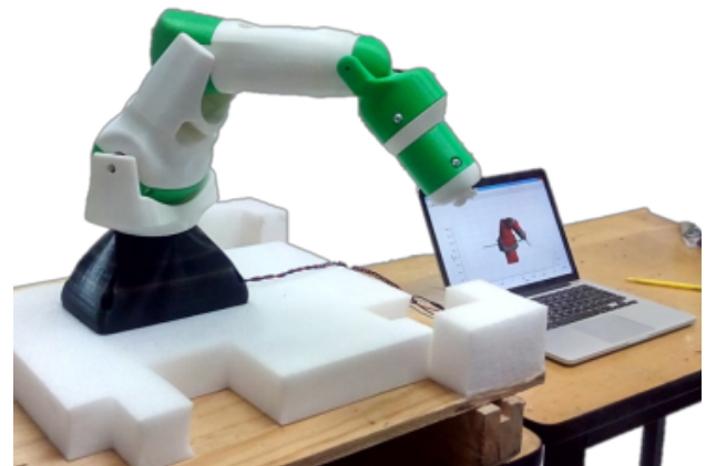
Fig. 6. Implementation of the 5 GDL anthropomorphic robot.
