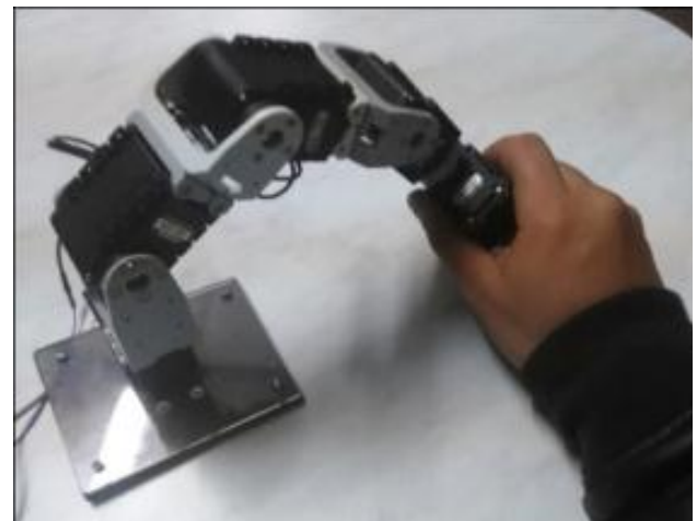
Fig. 23. Master robot implemented for teleoperation.
