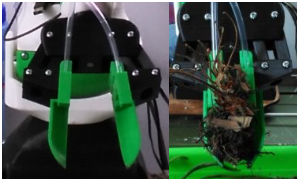
Fig. 7. End effector multifunctional and attachable.
