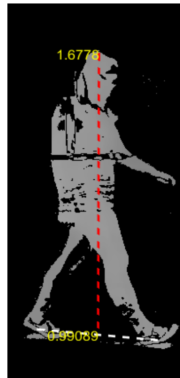
Figure 11. Real height and step length of a person obtained from depth image
