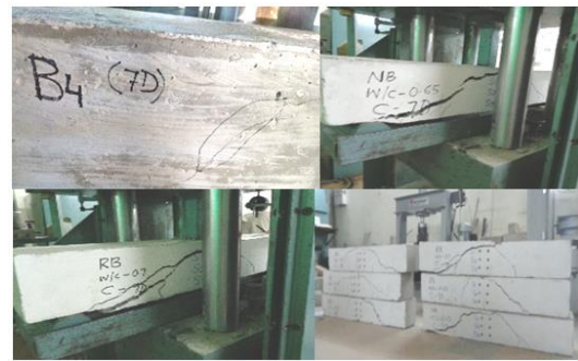
Fig. 9. Cracking in beams
