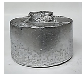
Fig. 2 Sample obtained after casting
