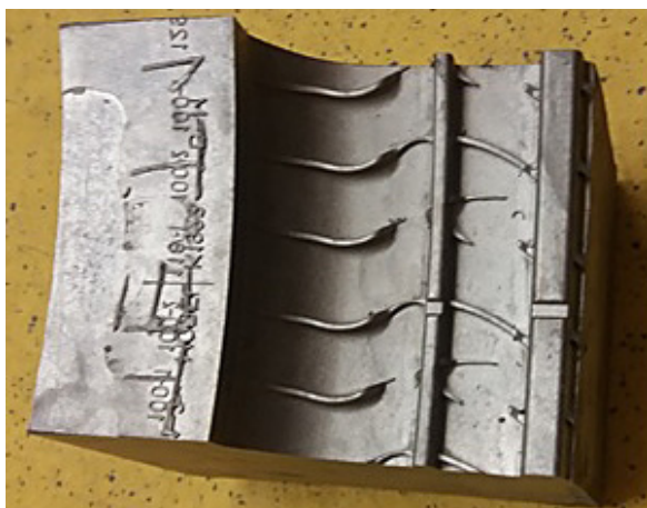
Fig. 1. Segment mold for tires production casted from aluminium alloy
