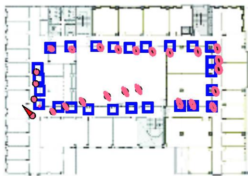
(a) Vanilla EKF-based SLAM. The E-dist of mapping is 1.70m.
