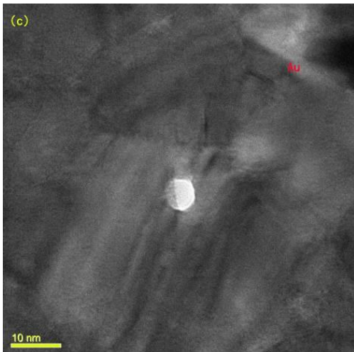
Figure 4. Nanopore drilled in the gold-covered region: (a) before drilling with a TEM magnification of 1000kX, (b) after drilling with a TEM magnification of 400kX, (c) after drilling with a TEM magnification of 800kX.
