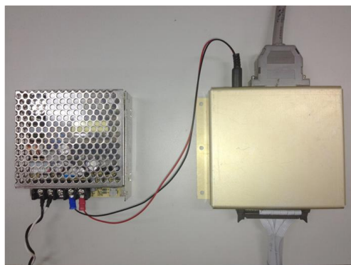
Figure 11. A power supply (left) and a driver (right).
