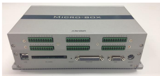
Figure 12. A real-time embedded controller (Micro-Box).
