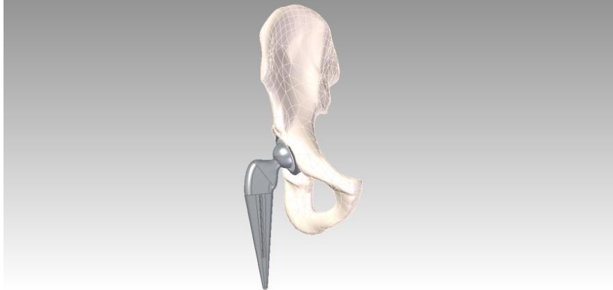
Fig. 4. The pelvic bone with mounted endoprosthesis of the hip joint (front view) [source: own study]
