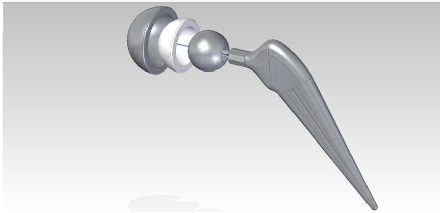
Fig. 3. The model of the endoprosthesis of the hip joint (extruded view) [source: own study]
