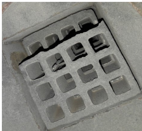
Fig 2b. Catalysts KP installed to lab SCR section
