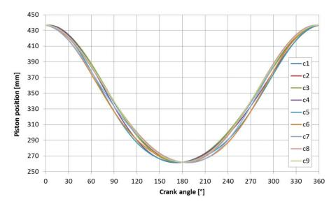
Fig. 5. Characteristics of position of the piston
