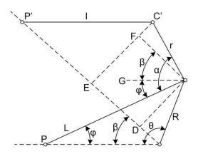
Fig. 2. Scheme of crank-piston system (Sibert, 1940)
