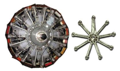
Fig. 1. AS-62IR engine and assembly of connection rods
