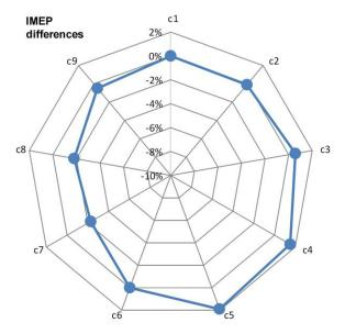
Fig. 9. Distribution of IMEP for each cylinder
