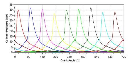
Fig. 8. Characteristics of pressure in the cylinders
