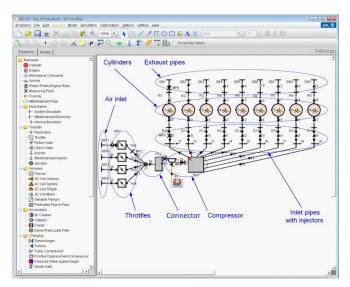
Fig. 4. 1D model of ASz-62IR engine (Pietrykowski & Gęca, 2014)
