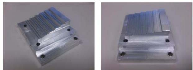
Figure 3. Designed ladder workpiece and fixture.
