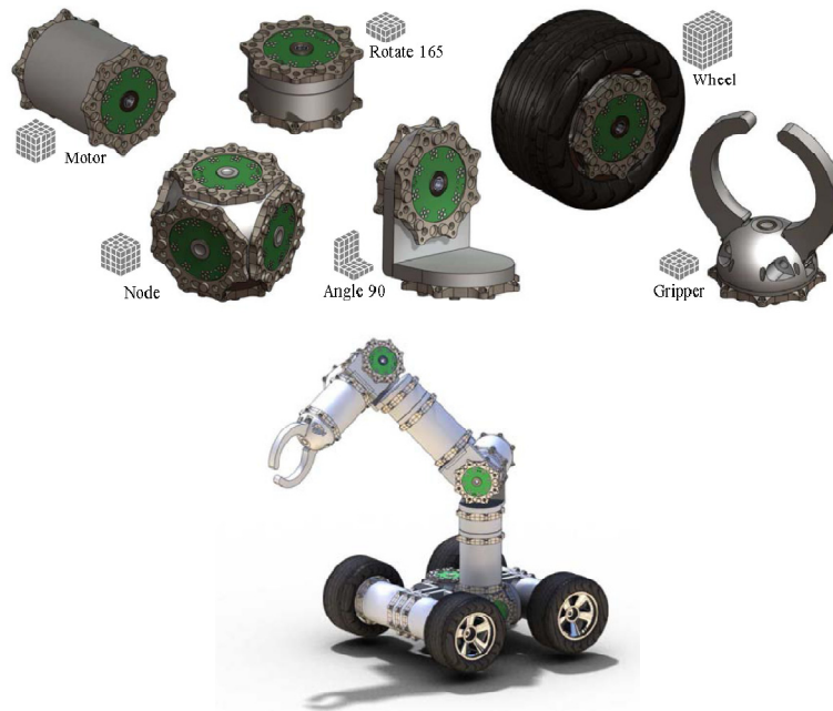
Fig. 6 Example of the possibility of reconfiguration of Thor model [source: own study]
