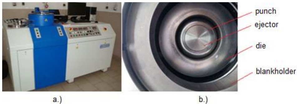
Fig. 1. a) universal testing machine Erichsen 145-60, b) tool set for deep drawing cup test [source: own study]
