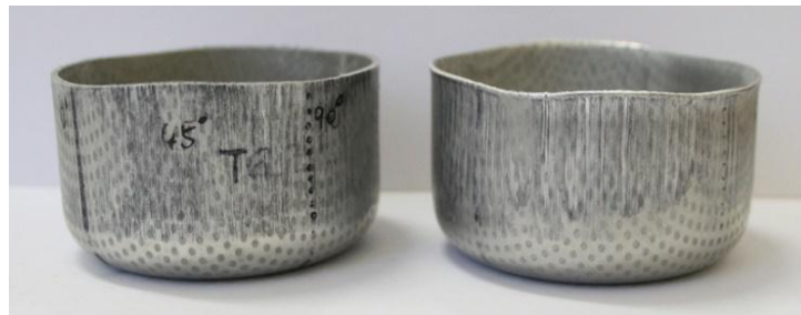
Fig. 4. Drawn cups from materials AW 6082 T6 (left) and AW 5754 H11 (right) [source: own study]
