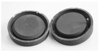
Fig. 4. Halves of the casting mold produced using FDM technology [source: own study]
