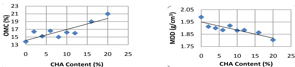
Figure 3 Variation in OMC and MDD with CHA content
