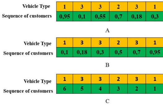
Fig 5-A. The proposed two-string representation before sorting the randomly generated the numbers in the second string Fig 5-B. The proposed two-string chromosome after sorting the randomly generated the numbers in the second string Fig 5-C. Proposed two-string chromosome with the sequenced customers
