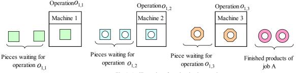
Fig. 1. An illustration of overlapping in operations
