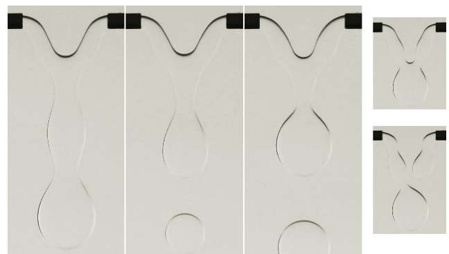
Fig. 5. Experimental observations of the breakup process for a mixture of 50% glycerin in water (frames separated by 166 ms). One can observe the multiple inflection points that the interface exhibits and the asymmetrical breakup of the upper meniscus.
