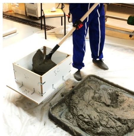
Fig. 1. Preparation of DPFC wall.
