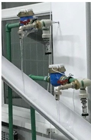
Fig. 2. Flowing water jets collected into the gutter channel.
