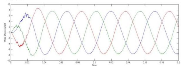
**Fig. 15.** Three Phase Currents of PMSM with ANN
