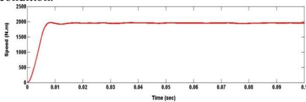
**Fig. 11.** Speed at 2000 rpm under no-load condition
