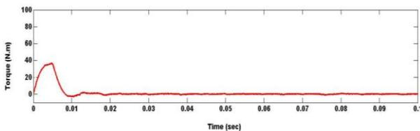
**Fig. 12.** Torque at 2000 rpm under no-load condition
