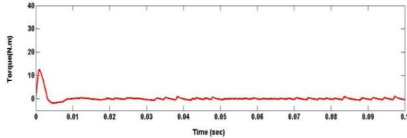
**Figure 10.** Torque at 1300 rpm under no-load condition
