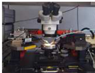
Figure 7. On-chip measurement station
