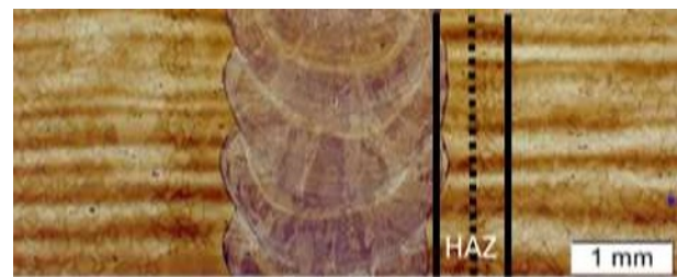
Fig. 8. Micrograph of a Laser-MPNG weld in Alloy 6170cc with a HAZ < 1 mm
