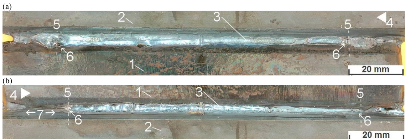
Fig. 9. Bottom view of optimized weld root (a)... 1 st pass (b)... 2 nd pass. 1... rail foot 2... weld pool backing inlay 3... weld root 4... welding direction 5... sidewise run-in/ run-out zones 6... TIG fixation weld spots 7... no root formation.
