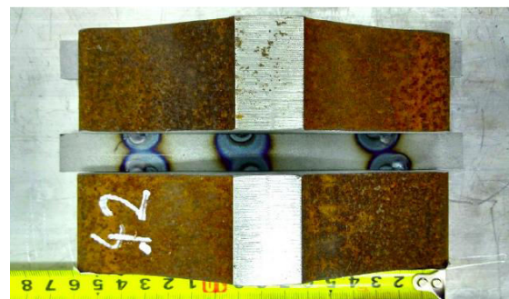
Fig. 2. Rail samples used for welding experiments.
