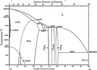
Fig. 4. Binary Al–Fe phase diagram [15].
