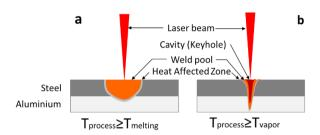
**Fig. 2.** Schematic representation of (a) conduction mode; and, (b) keyhole mode.
