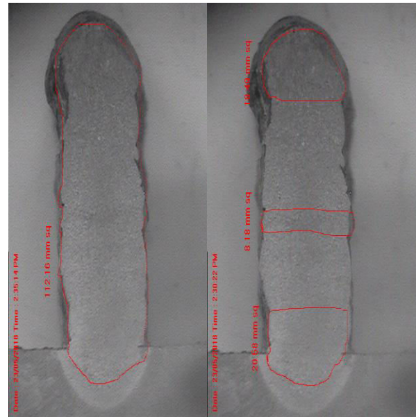
Fig. 8. Macrograph results of 10 layers WAAM experiment
