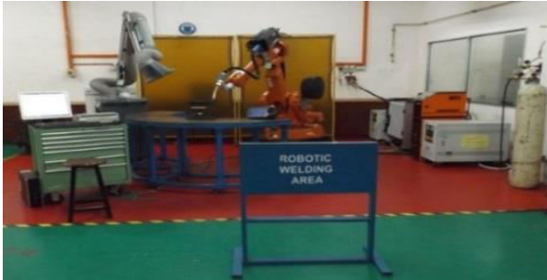
Fig. 7. ABB IRB 2400/16 Robotic welding Machine
