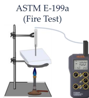
Figure 1. Experimental set-up of horizontal Bunsen burner fire test.
