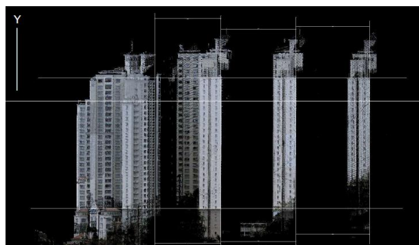
Fig. 13. Model of 4 tower of ASTON buildings along with X and Y axis to investigate the tilting
