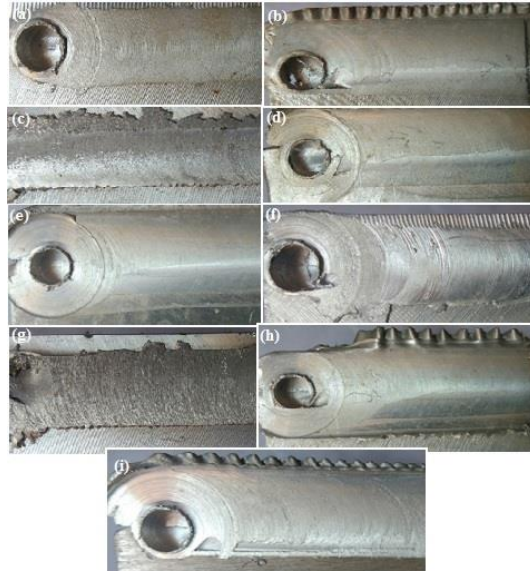
Fig. 4. Surface morphology of the welded specimens: (a) Experiment 1, (b) Experiment 2, (c) Experiment 3, (d) Experiment 4, (e) Experiment 5, (f) Experiment 6, (g) Experiment 7, (h) Experiment 8, (i) Experiment 9.
