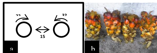
Fig. 2(a) An illustration of a gap and rotation of rollers in the bunch crusher and (b) spikelets of the oil palm bunch after crushed.
