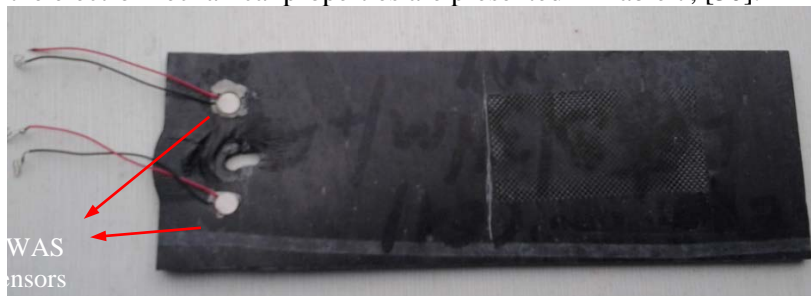
Figure 15. PWAS sensors positions on composite plate
