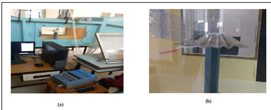
Figure 4. (a) Snapshot of experimental setup; (b) Corrugated A airfoil in wind tunnel
