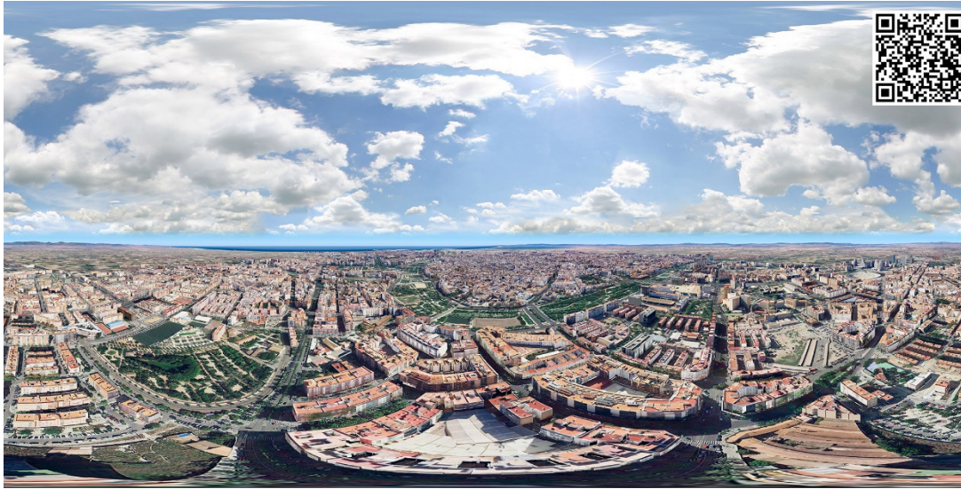
Fig. 11 - Equirectangular image composed using Hugin from the partial views obtained with Google Earth. The interactive visualization is available through the internet by reading the QR code in the figure with any mobile device
