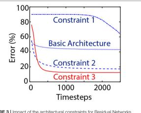
FIGURE 3 | Impact of the architectural constraints for Residual Networks. "Basic Architecture" does not involve any junction ReLU layers. "Constraint 1" involves junction ReLUs while "Constraint 2" imposes equal unity threshold for all residual units. Network accuracy is significantly improved with the inclusion of "Constraint 3" that involves pre-processing weight-normalized plain convolutional layers at the network input stage.
