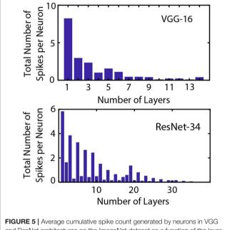
and ResNet architectures on the ImageNet dataset as a function of the layer number. Five hundred timesteps were used for accumulating the spike-counts for VGG networks while 2,000 time-steps were used for ResNet architectures. The neural spiking sparsity increases significantly as network depth increases.
