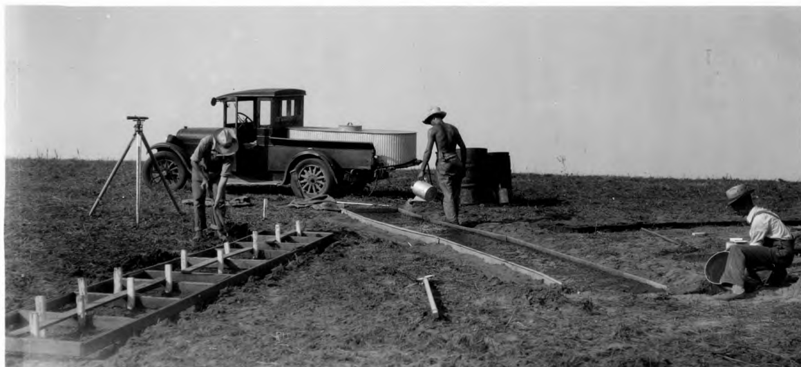
Fig. 1(b). Erosion measurements are being made on the plat at the right. This shows water being applied and the measuring of runoff. At the left a new plat with a different slope is being established
