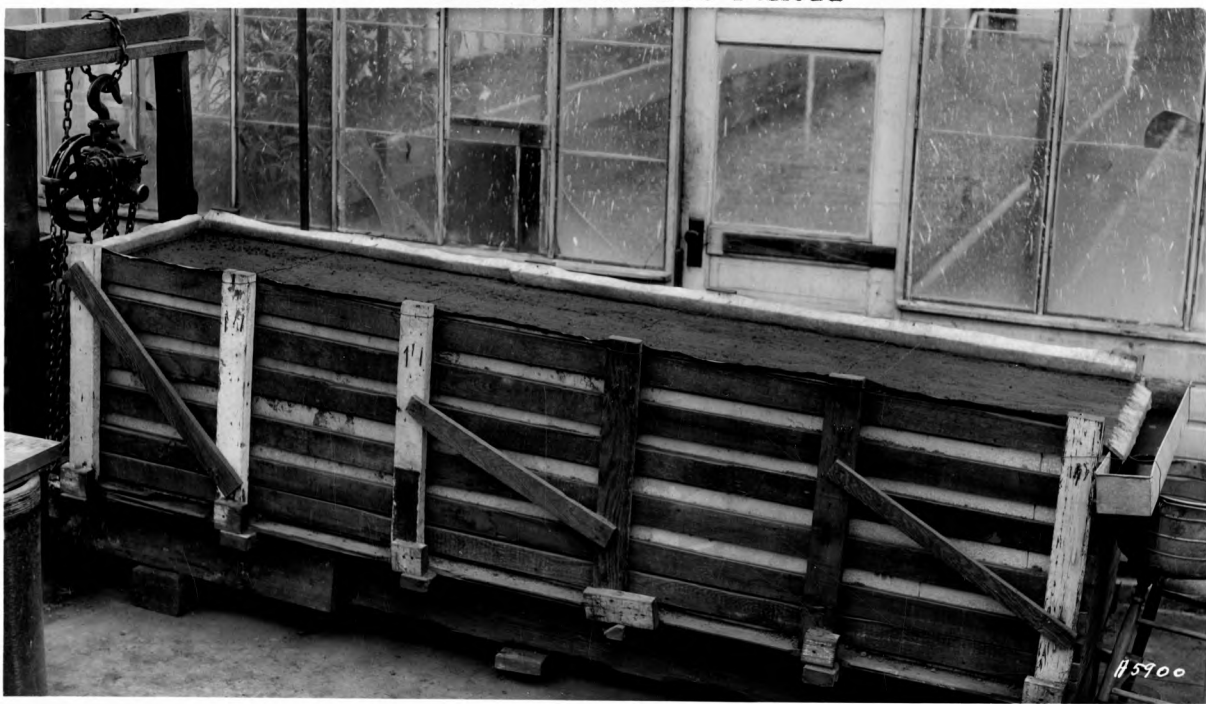
Fig. 2(a). Side view of tank used in erosion experiments. At left of picture is shown the differential hoist used to obtain different slopes
