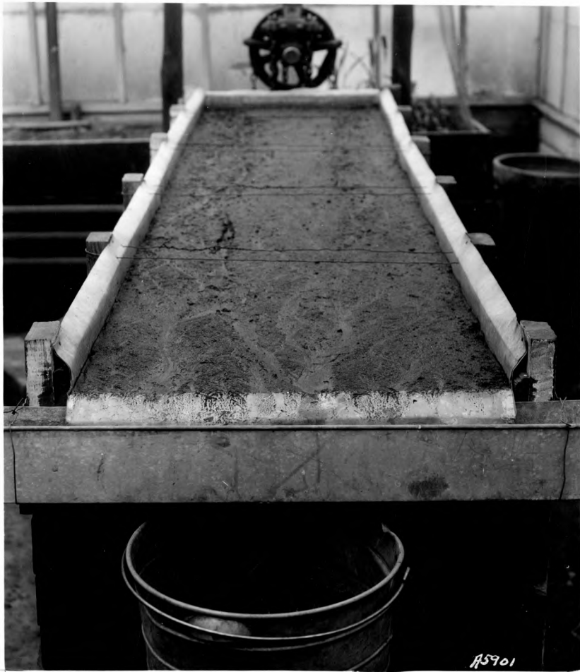
Fig. 2(b). Top view of tank showing method used to collect runoff
