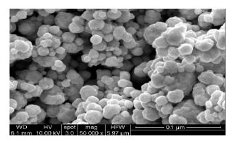
Figure 1: Real SEM Image of Nano Silver 20 nm.
