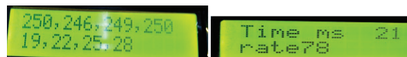
Figure 13. The Mode I display shows the four QRS peak values and the corresponding timings in ms. In mode II of display, it shows the total AP Propagation time and the heart rate.
