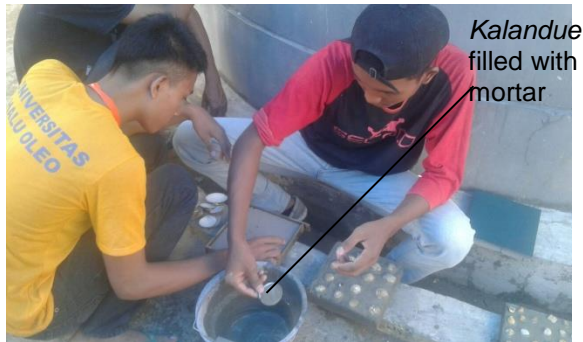
Figure 3. Kalandue shell filled with mortar
