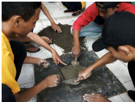
Figure 2. The bottom layer dough is pressed with a cement spoon
