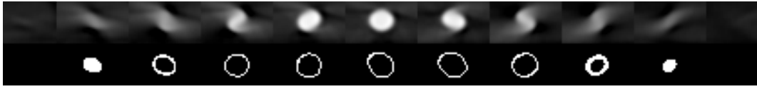
Figure 1: Cropped cone-beam CT volume of a metallic sphere (top row) and the result of performing 3D edge detection on the volumetric data (bottom row). Original image intensity values have been mapped to [0, 255] for display purposes. The filled circle edge images at both ends (left, right) of the sphere highlight the fact that the operation is indeed carried out in 3D. If performed on a slice by slice manner all edge images would result in empty circles.
