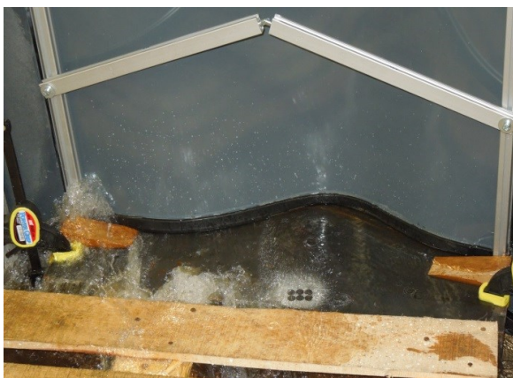
Fig. 5. Experimental measurement: hydrodynamic load of anti-flood board
