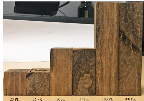
Fig. 1. Bamboo specimens used for compression tests – 25 mm, 50 mm and 100 mm height
