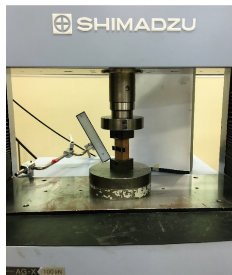
Fig. 2. Test set-up used for compression
