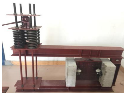
Fig. 4. Set-up of specimen in lever frame
