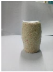
Fig. 6. Sample after tri-axial test (wood fiber concentration 0.03%)
