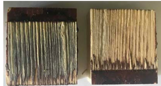
Figure 7. Shear failure surface of laminated wood
