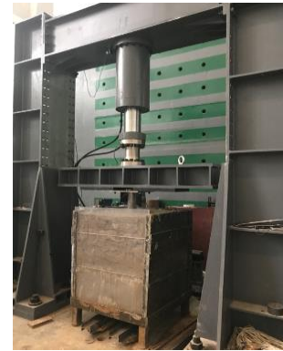
Fig. 12 Loading on the steel pipe pile
