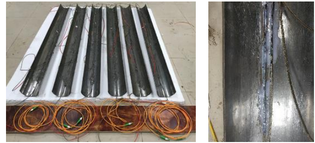
Fig. 11 The deployment of the Long-gauge FBG sensors
