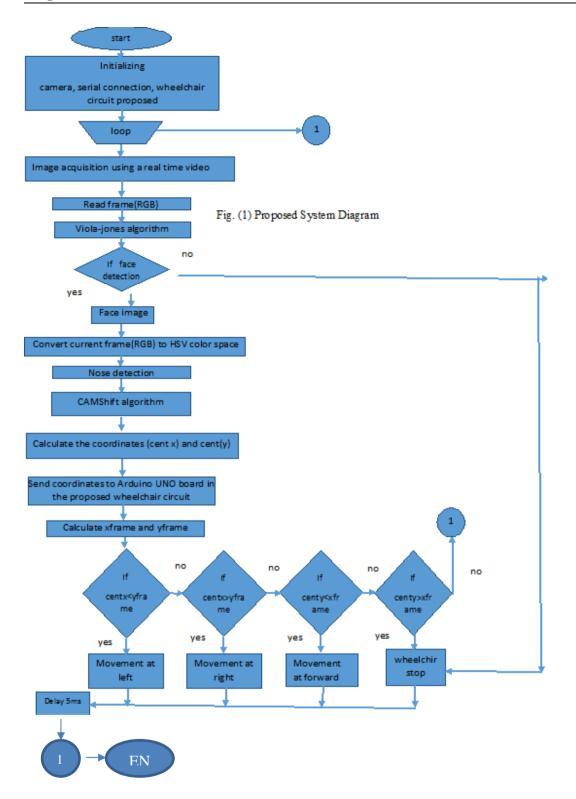
Fig. (2)Flowchart for Wheelchair Movement proposed
